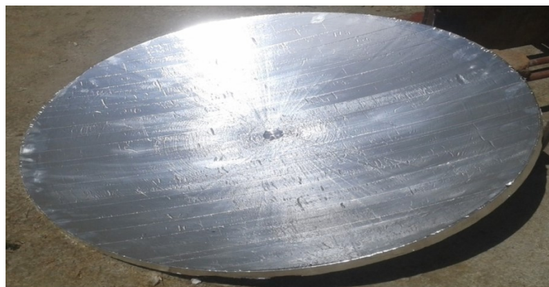
Figure 7. Appearance of a paraboloid with a foil-coated surface.
