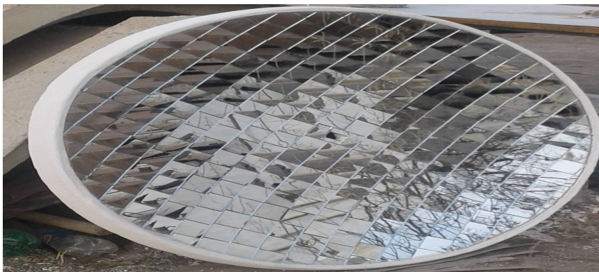
Figure 8. The surface is covered with mirrors 5x5 cm in size, the real appearance of the paraboloid.
