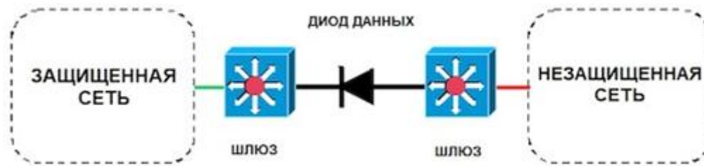
Fig 2. The simplest data diode application scheme.
